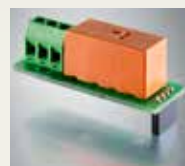
Releu conectare lumini garaj
